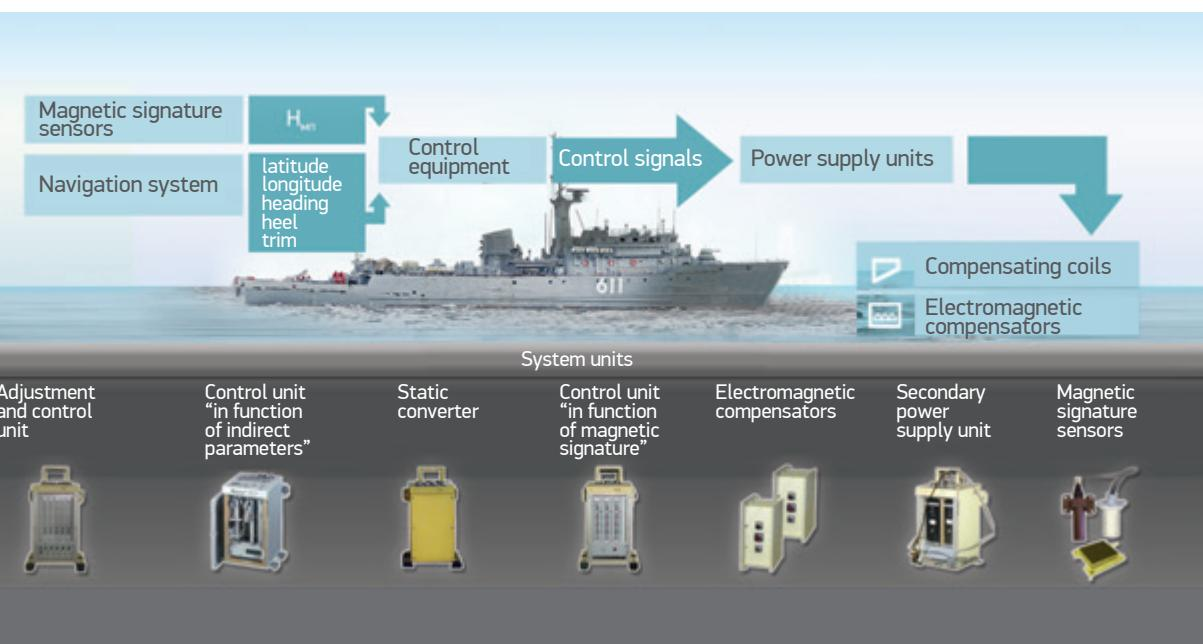
On-board degaussing KDS systems are intended for automatic regulation of currents in degaussing coils of surface ships. Application of these systems provides automatic compensation of magnetic field and, accordingly, reduces the ship's magnetic signature.
